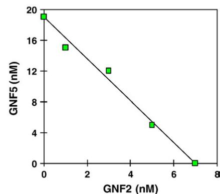
**Fig. 3.** Additive effects of increasing concentrations of GNF-2 and GNF-5 on the kinase activity Abl64–515. Isobologram analysis showing simultaneous exposure of Abl64–515 to increasing concentrations of GNF-2 and GNF-5. Starting concentrations were 10  $\mu\text{M}$  for each compound with 3 step dilutions down to 0.003  $\mu\text{M}$ . Isobologram analysis was performed as described in Experimental procedures.
